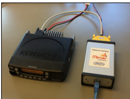
Network Interface connected to Kenwood NX-720
