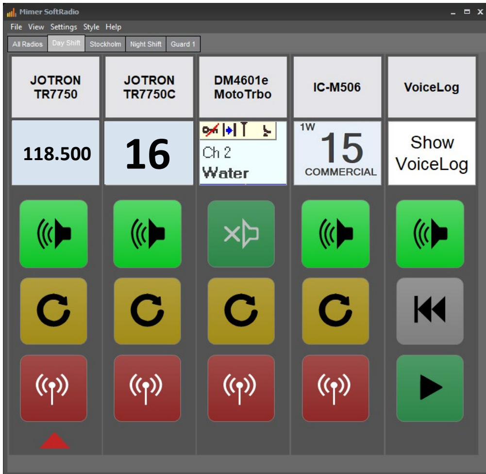
Example of SoftRadio with both Marine and Airband radios plus DMR and a VoiceLog
