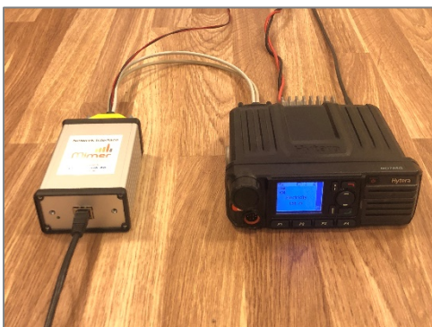
Network Interface connected to Hytera MD785
