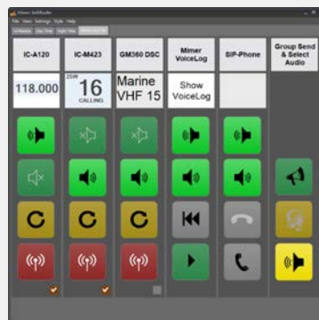
Mimer SoftRadio with three radios, voice log and SIP phone connected
