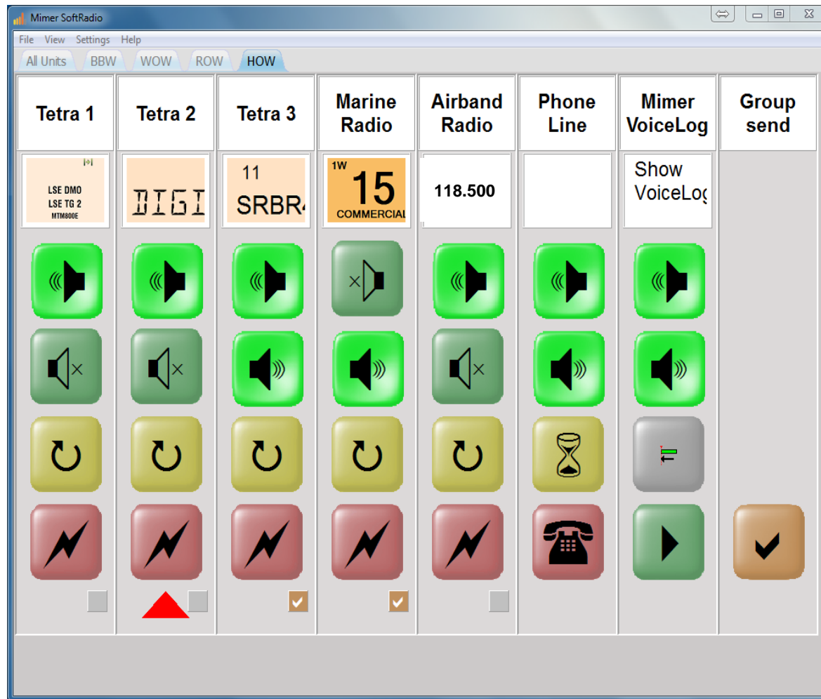
Example of SoftRadio GUI Tetra+Marine+Airband+Phone
