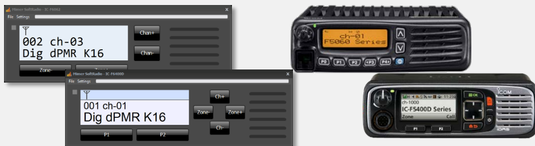
Virtual Control Heads for the Icom F5060 and F5400 shown to the right
