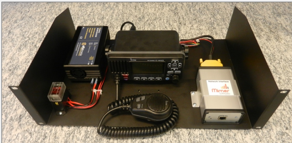
Icom marine radio installed on a 19" 3U shelf
