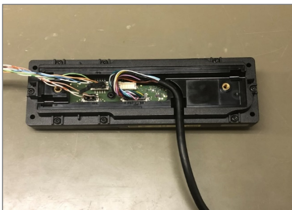
Backside of control head
