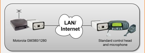
Example of set up with radio and control panel separated
