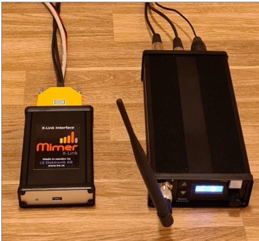
Vokkero “WI” connected to a X-Link interface
